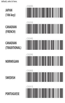
IntelliScanner emulates a keyboard. If you're using a keyboard layout other than the
